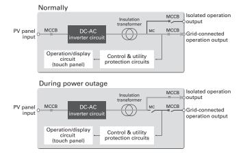
Fig. 2: A block diagram of an isolated operation circuit
