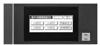
Fig. 6: Utility protective function setting screen of the "SANUPS P83E" touch panel
