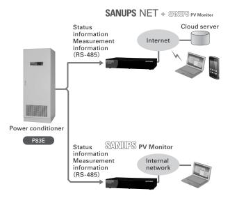
Fig. 3: An example of remote monitoring
