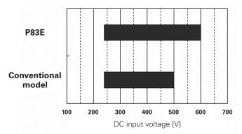
Fig. 1: Comparison of input operating voltage range
